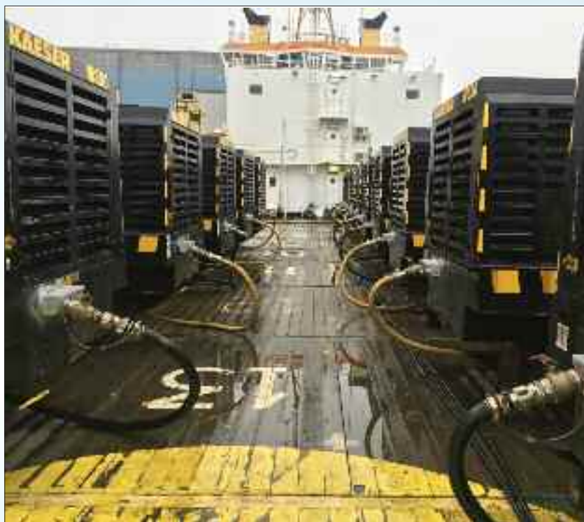
Bodac bubble curtain aircompressors mammal mitigation.
